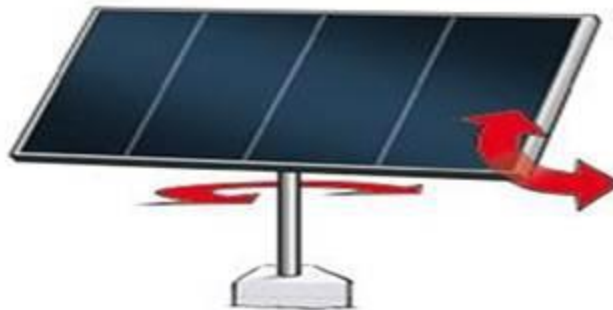
Figure 2.5.2 Tip-Tilt Dual-Axis Solar Tracker [27]
