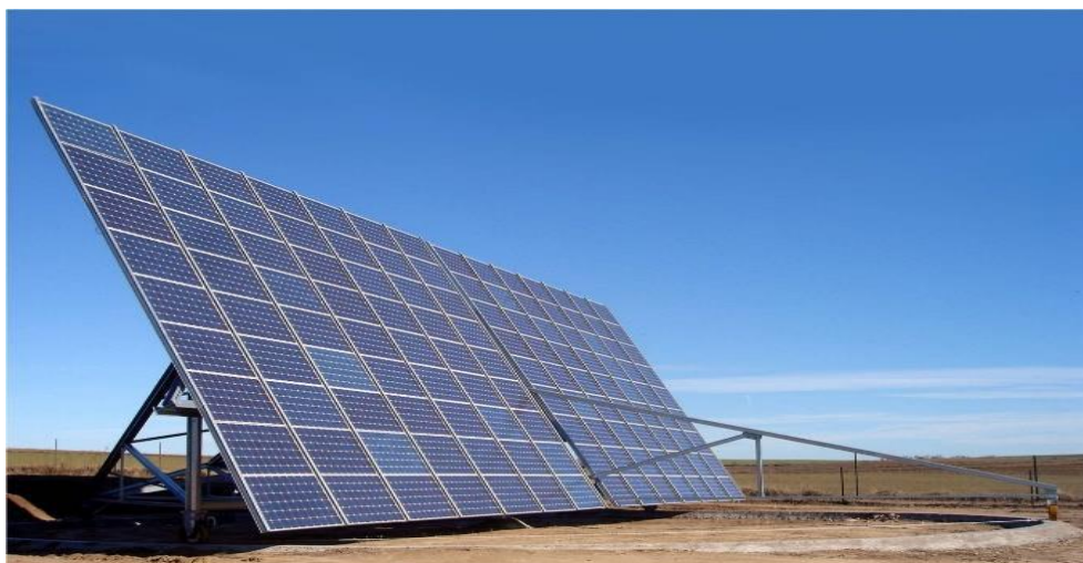
Figure 2.5.3 Azimuth-Altitude Dual-Axis Solar Tracker [28]
