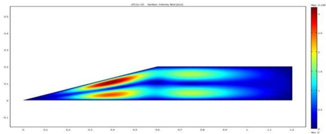
**Fig. 2(a):** Shows the Velocity field distribution when the enclosure was heated from the base walls at  $18^\circ$ -pitch,
