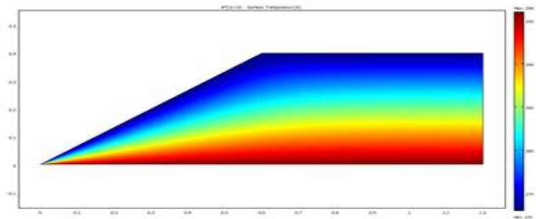
**Fig. 4:** shows the mean temperature distribution within the enclosure at 30<sup>0</sup>-pitch, isothermally heated through isothermally cold through the inclined wall,  $Ra=2.31 \times 10^6$ .
