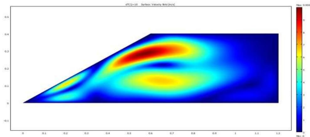
**Fig. 2(b):** Shows the Velocity field distribution when the enclosure was heated from the base walls at  $30^\circ$ -pitch,
