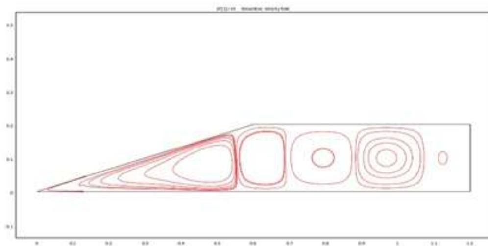
**Fig. 3(a):** Streamlines of the enclosure heated below at 18°- pitch,  $Ra=1.57 \times 10^5$ ,  $AR=0.3$
