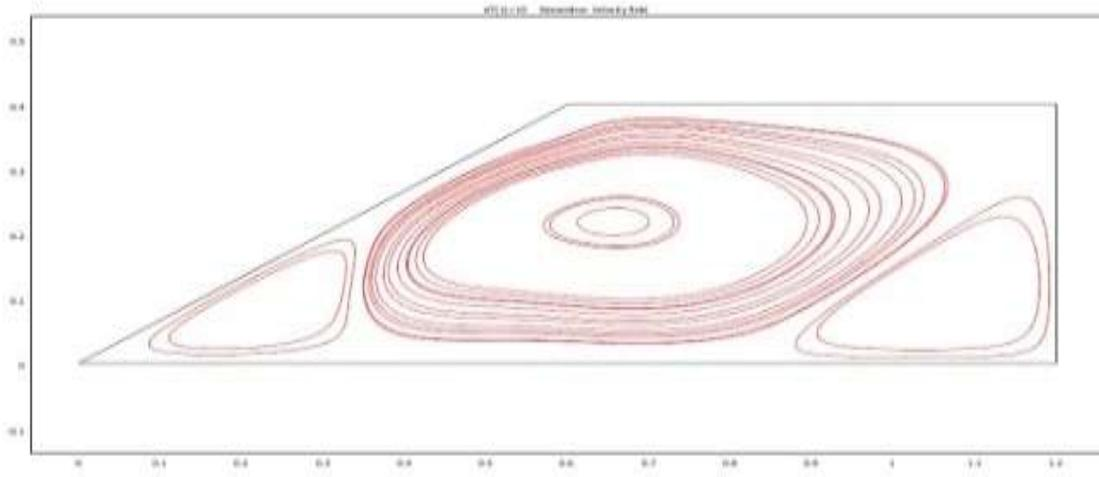
**Fig. 3(b):** Streamlines of the enclosure heated below at  $30^{\circ}$ - pitch,  $Ra=5.41 \times 10^5$ ,  $AR=0.3$
