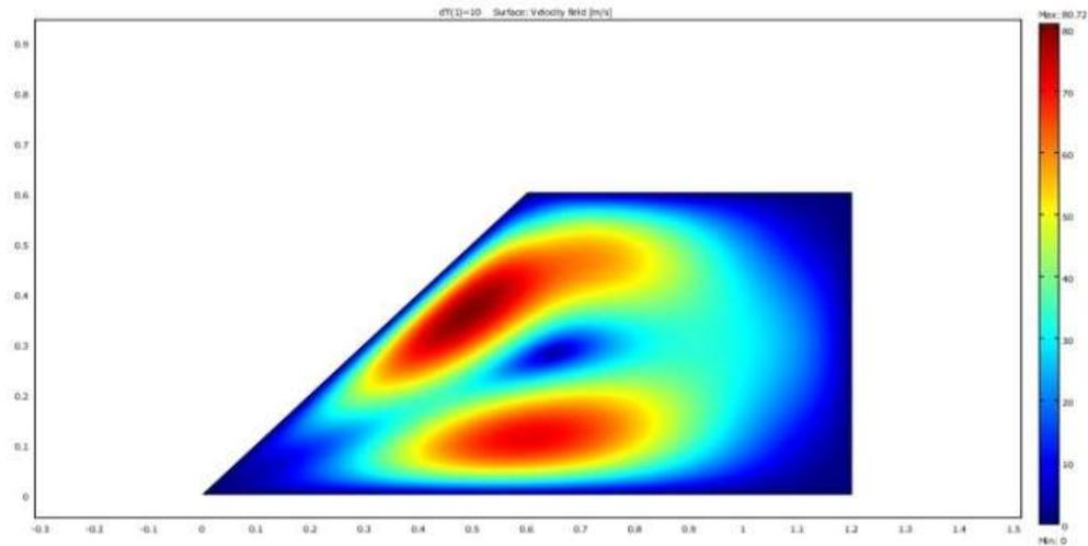
**Fig. 2:** Shows the Velocity field distribution when the enclosure was heated from the base walls at 45°-pitch.
