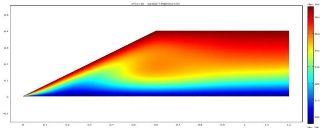
**Fig. 4(a):** Shows the mean temperature distribution within the enclosure at 30<sup>0</sup>-pitch, isothermally heated through the inclined walls  $Ra=2.50 \times 10^6$
