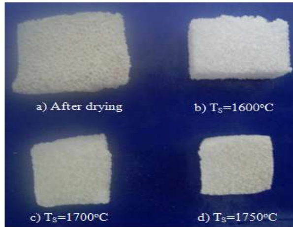
Fig. 3: The image of alumina-based foams after drying and heat treatment
