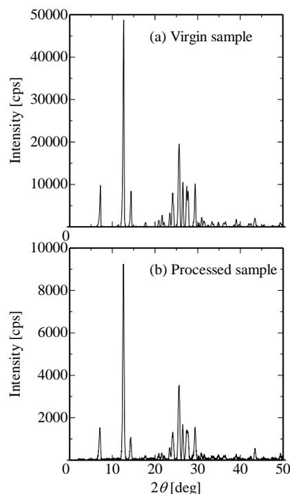
**Fig. 8** XRD patterns of theophylline; (a) virgin particles, and (b) particles produced.
