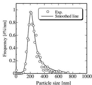
Fig. 6 Particle size distributions (PSD) of processed theophylline particles.
