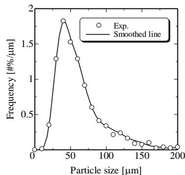
**Fig. 3** Particle size distributions (PSD) of virgin theophylline particles.
