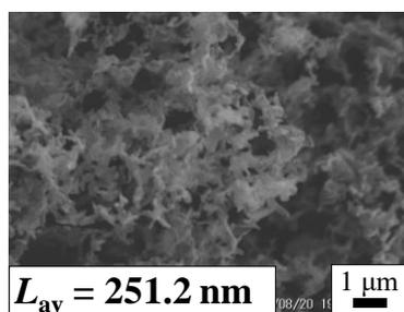
Fig. 5 SEM photograph of processed theophylline particles.
