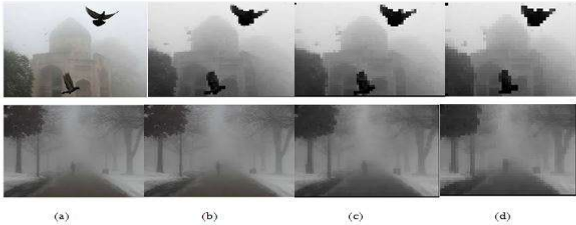
Fig.3 Dark Channel of Various size (a)Hazy Image Dark channel prior with patch size of (b)3*3 (c)7*7(d)11*11
