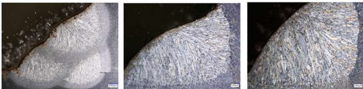
Figure 3 Macrostructures of welded joints in protective shielding atmospheres: Ferroline C18 (left), Ferroline C6X1 (middle), Ferroline He20C8 (right)
