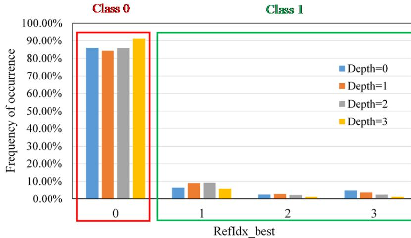
Fig. 4. Frequency of occurrence of best reference frame index (RefIdx\_best).
