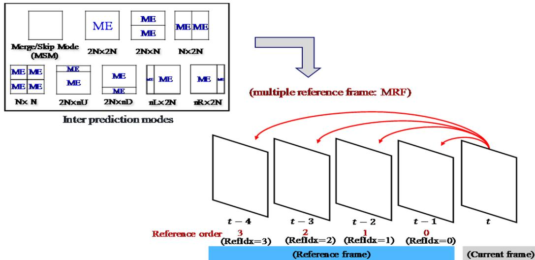
Fig. 2. The selecting process of inter prediction mode using MRF scheme.
