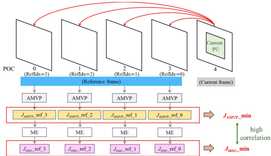
Fig. 3. The encoding process of MRF-ME on H.265/HEVC using four reference frames.
