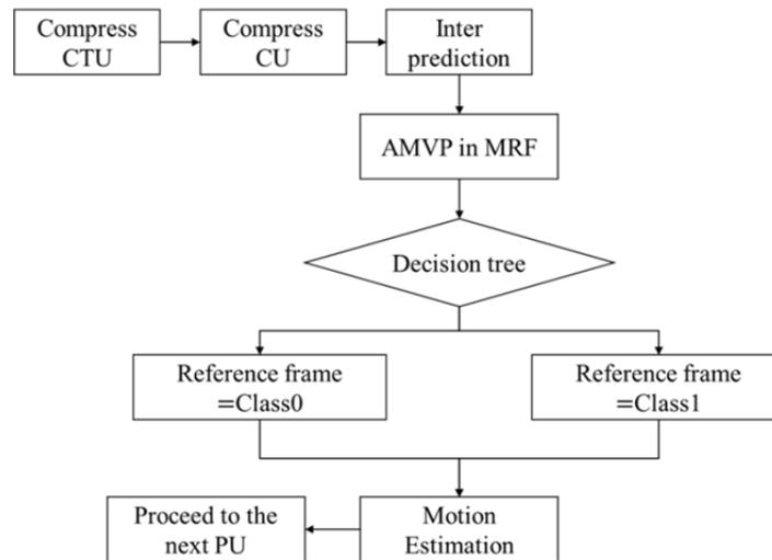
Fig.11. Flowchart of the proposed fast multiple frame selection.
