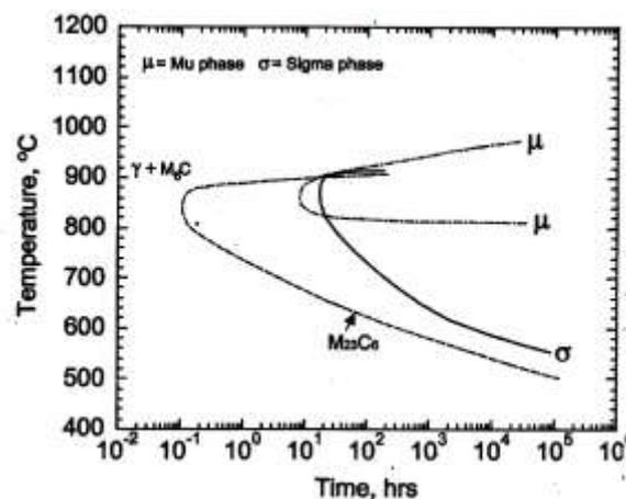
Fig. 6: Phase Precipitation and Time- Temperature Transformation Diagram of Hastelloy X [13]
