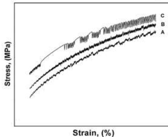
**Fig. 4: Schematic Representation of Different Types of Serrations**
