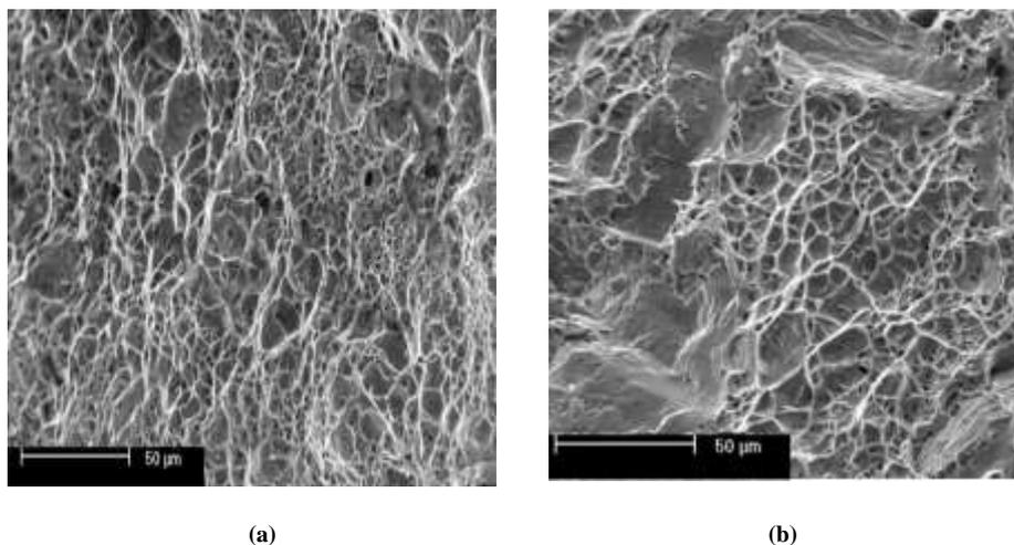
**Fig. 5: Fracture Surfaces of Tensile Specimens Tested at (a) RT (ductile mode of failure) at strain rate of 10-3 s-1 and (b) 650°C (mixed mode of failure) at strain rate of 10-5 s-1**
