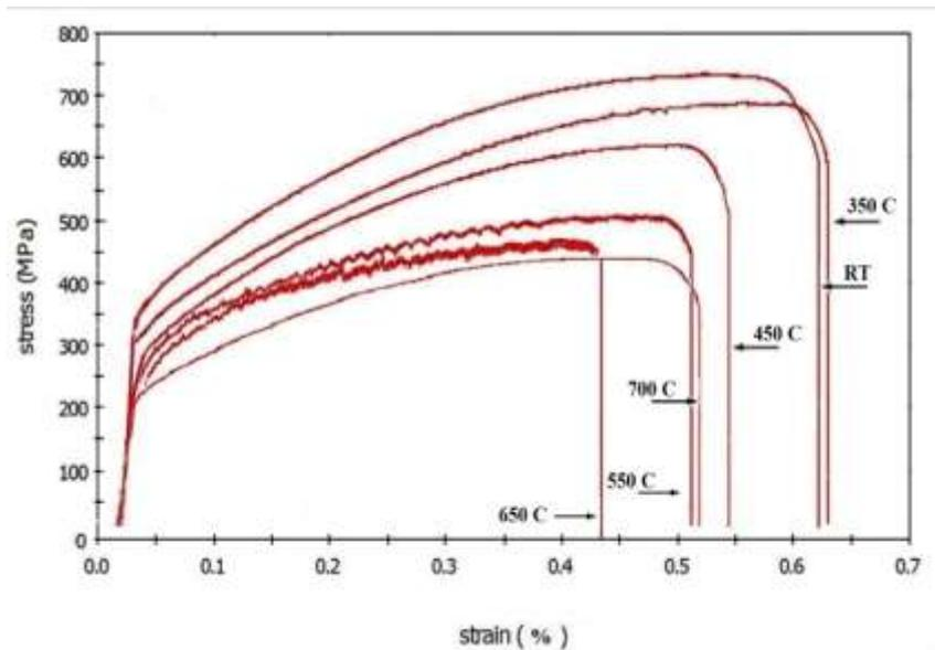
**Fig. 1: Stress- Strain Curves at A Strain Rate of 10-3 s-1 at Various Test Temperatures**
