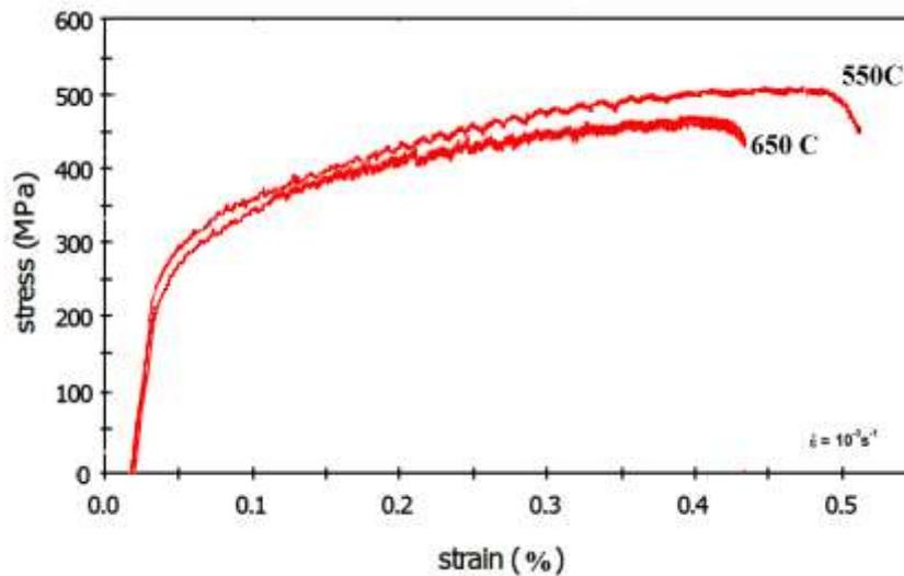
Fig.2: Stress-Strain Curves of Hastelloy X Tested at 550 And 650 °C at A Strain Rate of 10-3s-1
