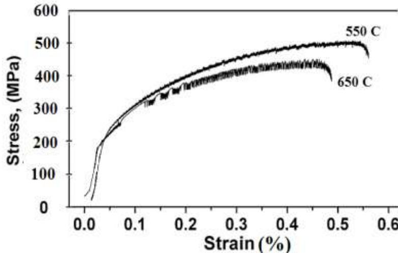
Fig.3: Stress-Strain Curves of Hastelloy X Tested at 550 And 650 °C at A Strain Rate of 10-5s-1
