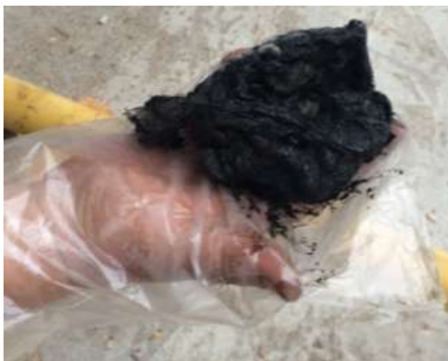
Fig.4 Condition of fabric filter placed in gas line after 20 minutes of operation of gas generator without a cleaning system
