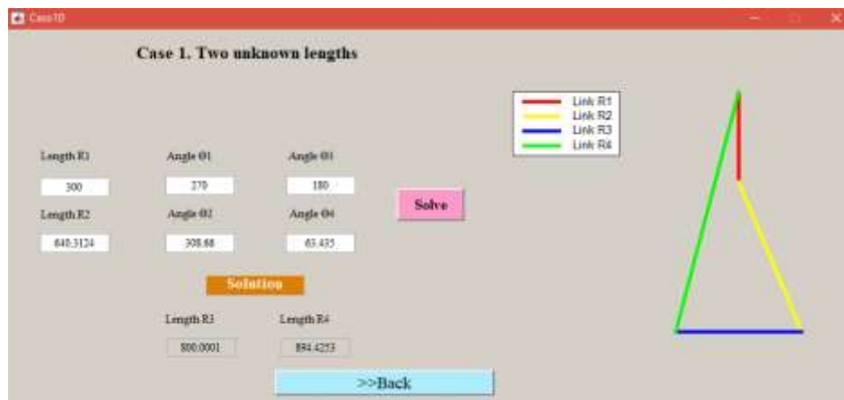
Figure8. Window of calculation and results in the analysis of position of a four-bar mechanism
