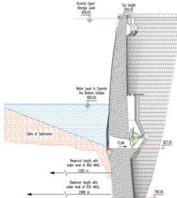
**Principle-** If the water level is reduced, the reservoir is full with sediment laden water. If as such the sluice gate is opened there will be discharge of the sediments. However the reduction in water level causes loss of water. Therefore, drawdown and sluicing time must be minimized.
