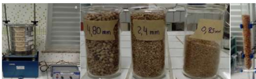
Figure 1: Construction of the granular filtration system. Initial mechanical separation of the sand collected in river bed (a); details of the granulometric fractions used in the construction of the filters (b) and assembly of the filter column (c).
