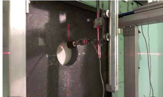
Fig. 4: The {}^6\text{Li} + Si detector in the holder.
