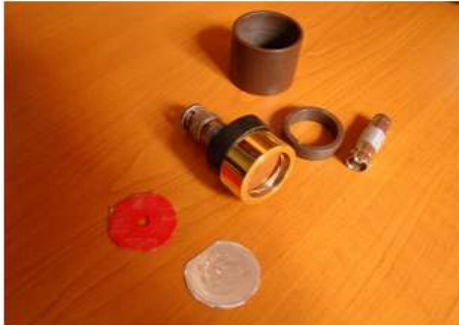
Fig. 3: The {}^6\text{Li} + Si detector.
