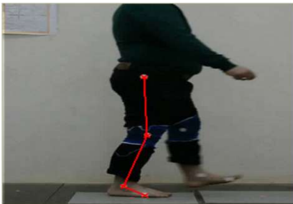
Figure 4: Marker's positions being digitized during a subject walking trials.
