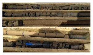
Figure 7: Images of some Drill Core Samples in core trays from Onupi Coal Mine.
