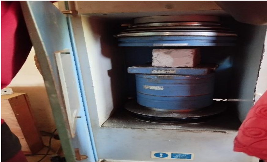
Figure 1: Testing Machine Compressive Strength Set up
