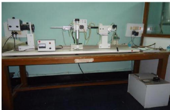
Figure 2: Leitz Heating Microscope
