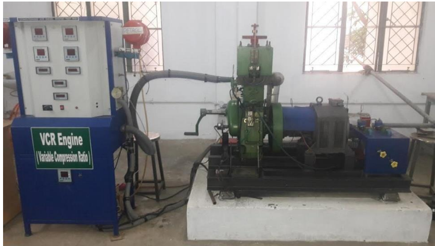
Figure2 Variable Compression Ratio Multi Fuel Test Engine
