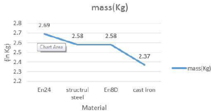
Figure 3: Variation of Weight of Camshaft of Different Materials
