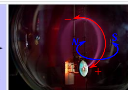
Beam of electrons moving in a circle, due to the presence of a magnetic field. Purple light revealing the electron's path in this Teltron tube is created by the electrons colliding with gas molecules.
