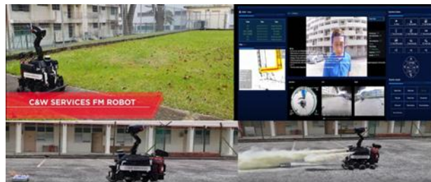
Figure 3: Application of FM Robots in Building Operations (Surveillance and Fire-Fighting Operations)
