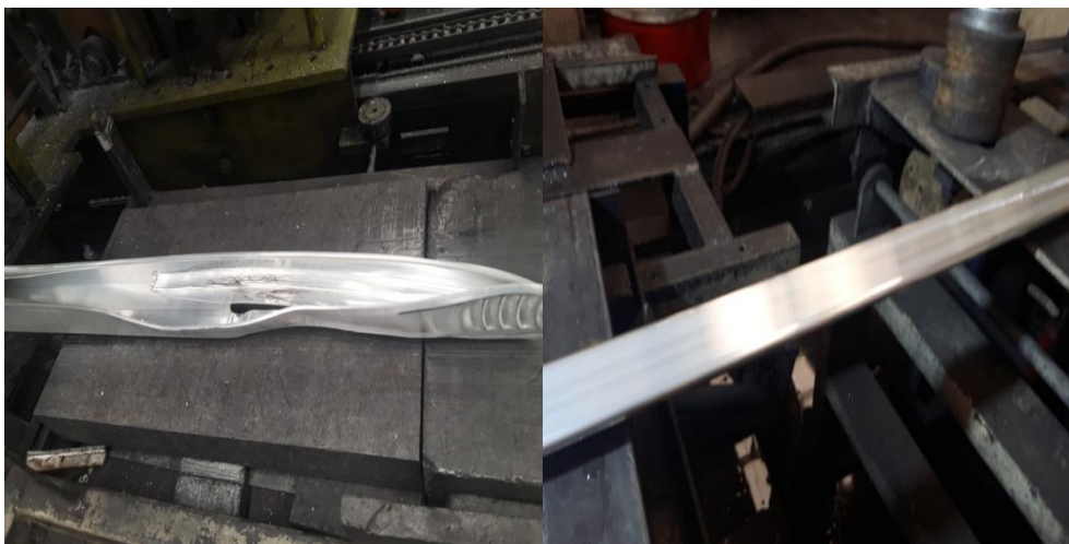
Figure 6. The extrusion process of sample 1 (left) and 2 (right)
