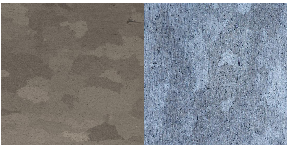
Figure 4. The microstructure of homogenized sample 1 with 480 °C (left) with 8 hour and 480 °C (right) with 10 hour
