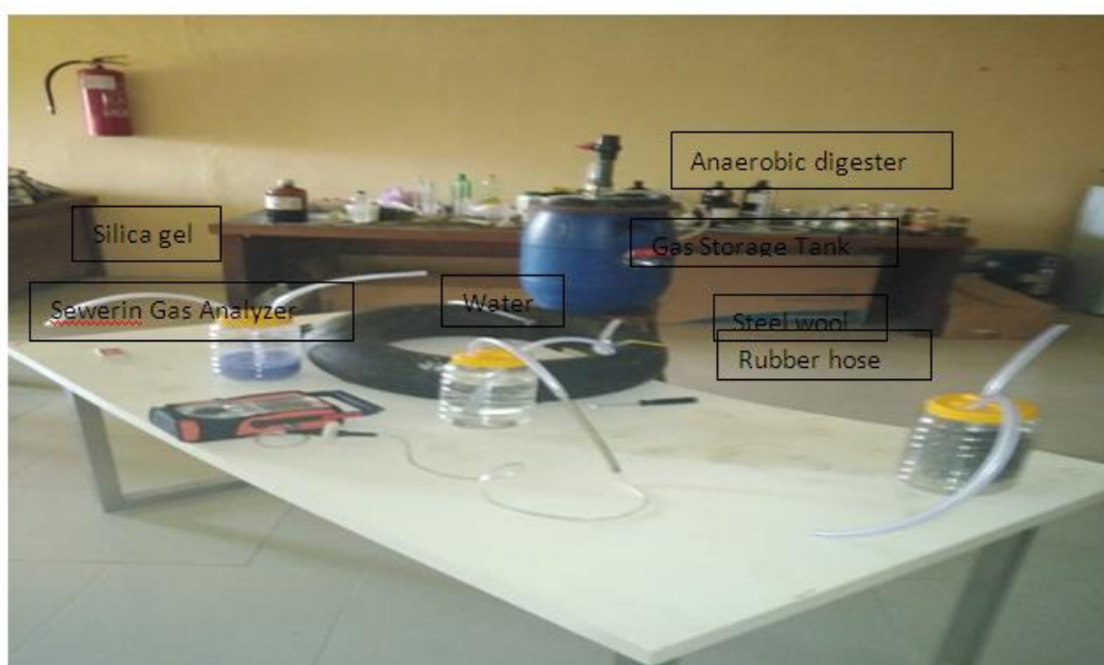
Plate (3): of Biogas Purification Set-up
