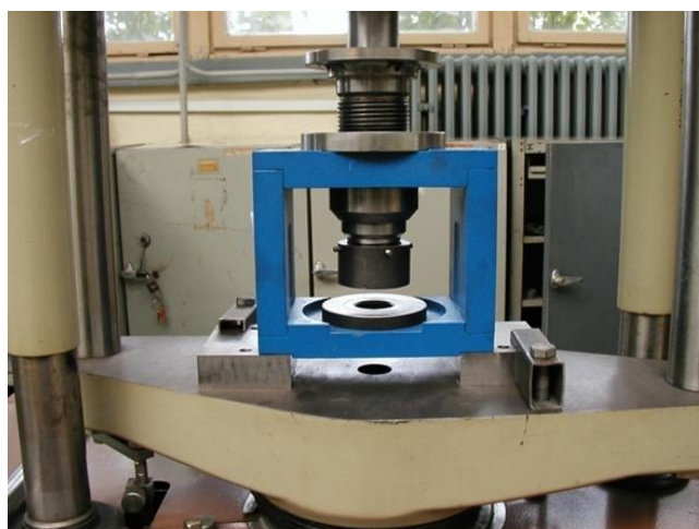
Figure 1 Deep-drawing tool for cup test
