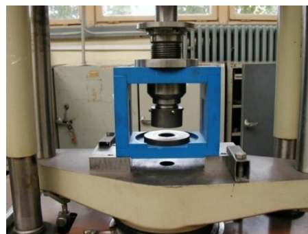
Fig. 1 Tool for cupping test
