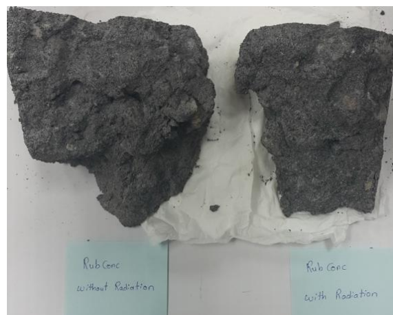
Fig.8: Rubberized Concrete Failure Surface. Left image represents the un-irradiated crumb rubber used while the right image represents the irradiated one
