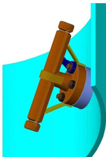
**Figure 02:** Drawing of the layout of the flow distributor separator vessel.
