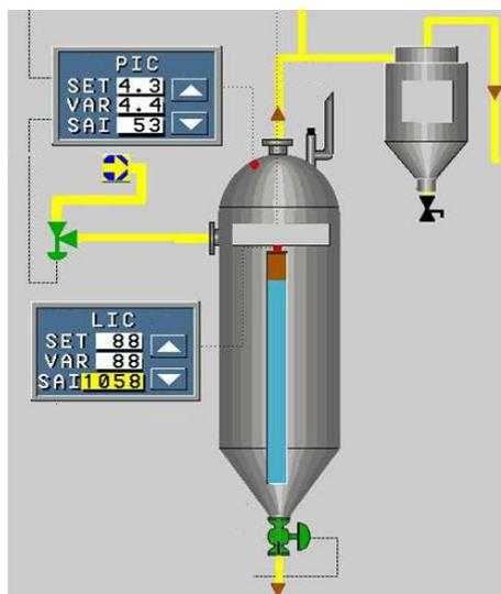
Figure 06: Indication of level control on the screen of DCS.
