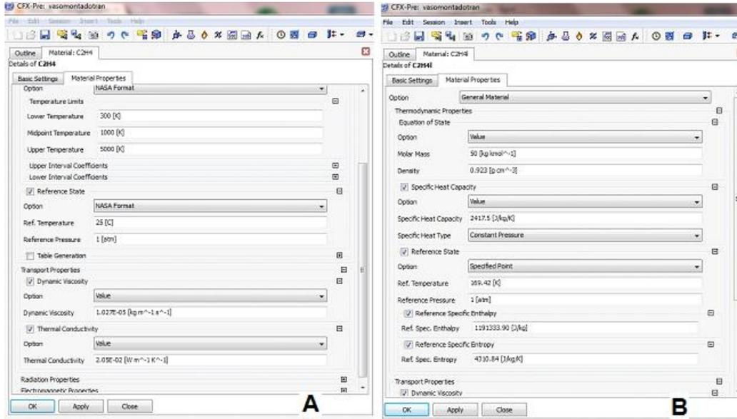
**Figure 03:** Screenshot of the software with the physical properties of the fluids and constants: The gaseous ethylene and LDPE liquid B.
