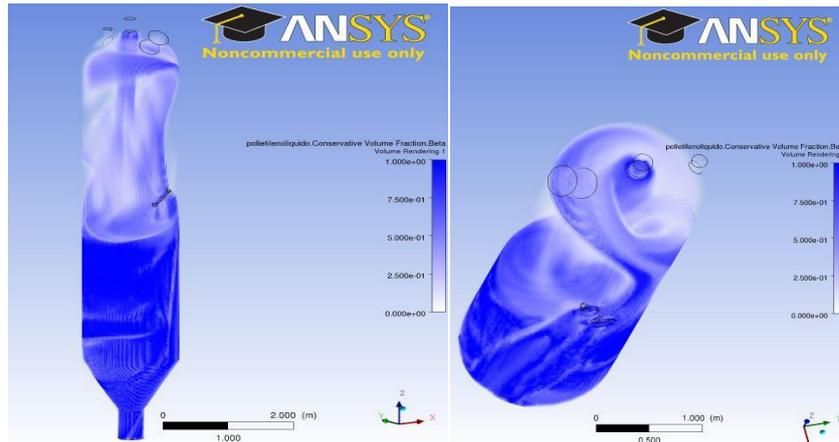
Figure 05: Map of separation of the two materials in the fluid in its liquid form is represented with blue color and gaseous blank. In the front view, and B in perspective showing the manhole and higher output.
