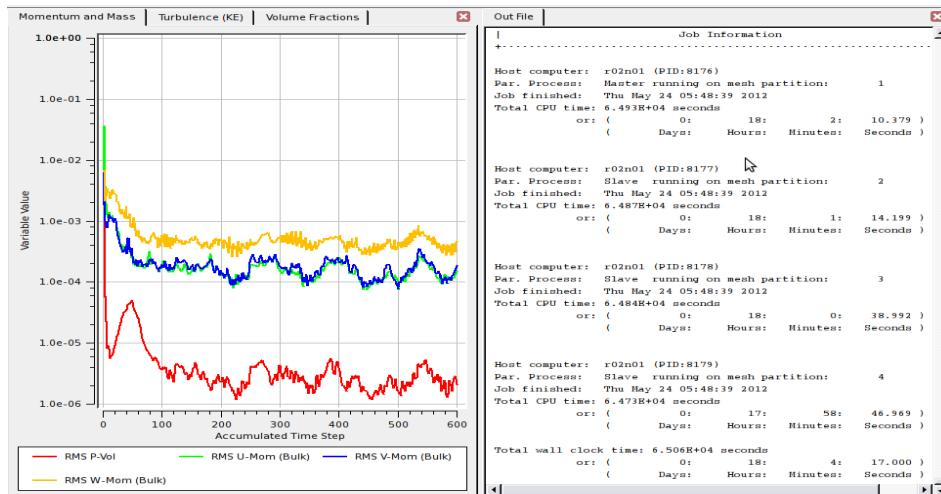
Figure 05: Convergence results for the moments of mass coordinates and corresponding processing time.
