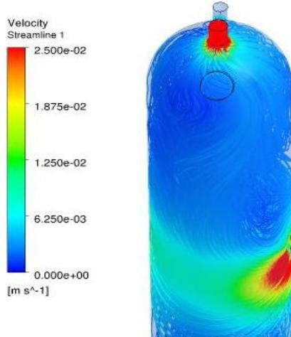
**Figure 07:** Lines of flow velocity of the fluid at the top of the vessel.
