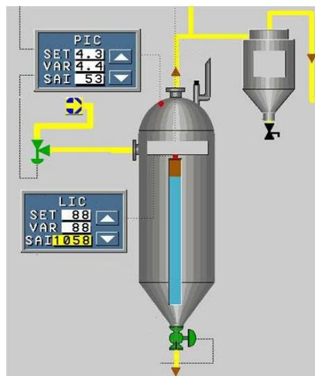
**Figure 06:** Indication of level control on the screen of DCS.
