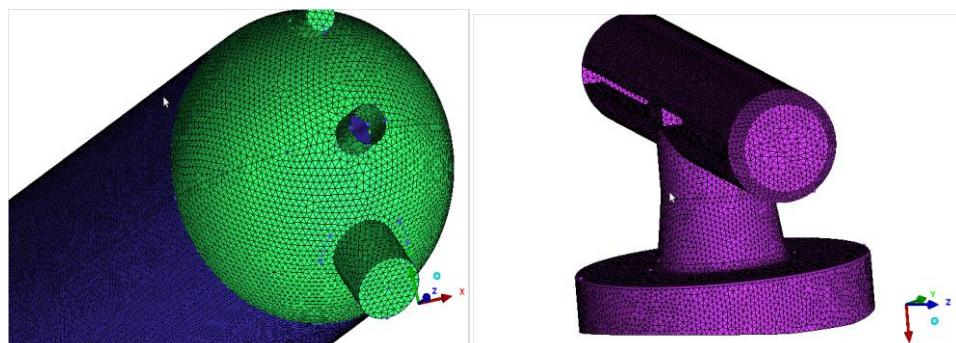
**Figure 04:** Tetrahedral mesh used in the numerical solution (separator vessel in distributor A and B).
