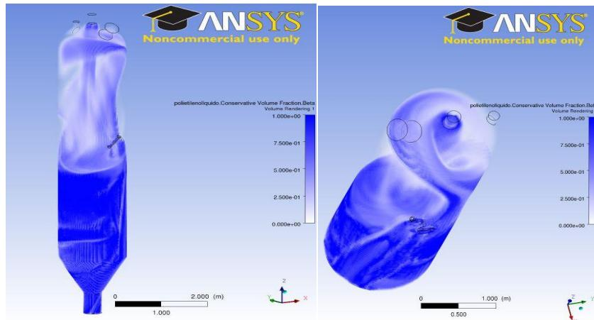
**Figure 05:** Map of separation of the two materials in the fluid in its liquid form is represented with blue color and gaseous blank. In the front view, and B in perspective showing the manhole and higher output.
