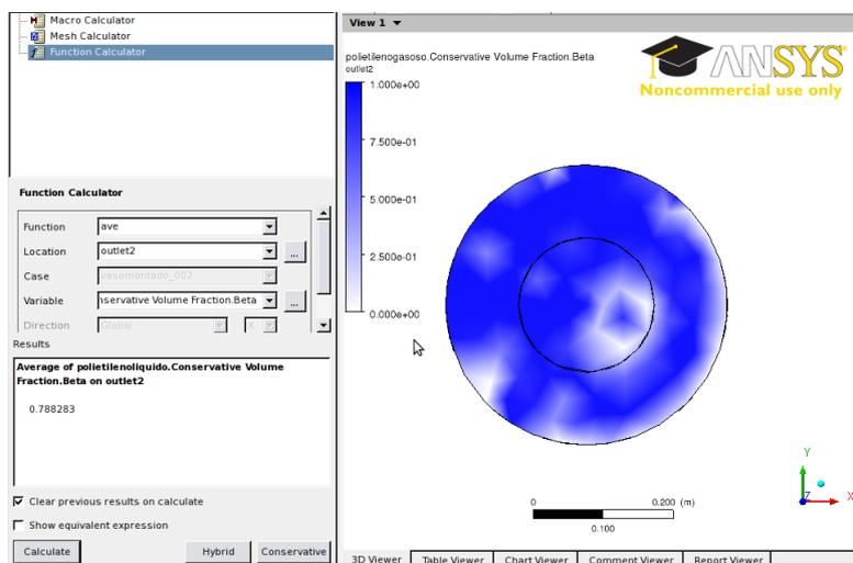
Figure 06: Calculation% of resin (blue) in the bottom outlet of the vessel.
