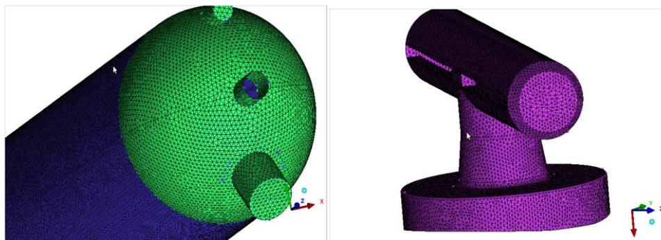
**Figure04:** Tetrahedral mesh used in the numerical solution (separator vessel in distributor A and B).
