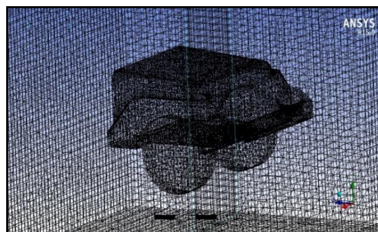
Fig. 6. Detailed view of bumper assembly mesh
