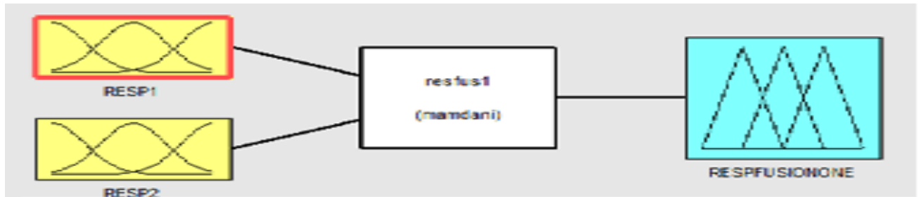
Figure 3.5: Basic FIS Editor in Matlab showing RESP1 and RESP2 outputs fused linearly to produce RESPFUSIONONE into a fuzzy model.
