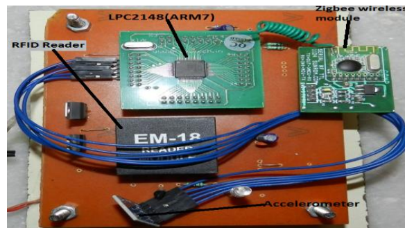
Fig. 3 Prototype of wearable sensor device of Transmitter side
