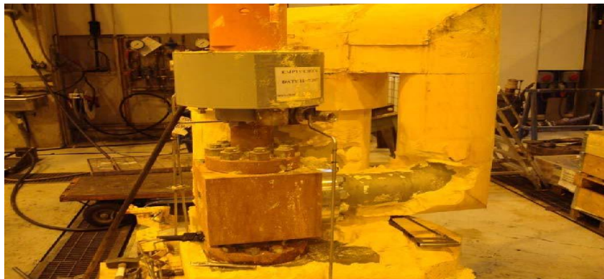
Figure 7: Sand accumulation in surface equipment.
