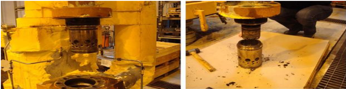
Figure 9: Sand accumulation effect on surface choke
