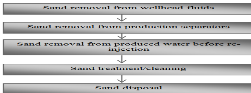
Figure 1: sand management equipment brake down processes
