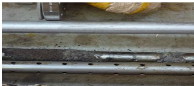
Figure 8: Sand accumulation effect on tubing
