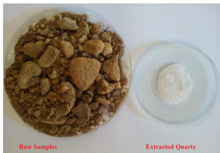
Figure 3: The raw sand samples collected from the terrace of Thoubal River at Leirongthen at depth 6 feet and the quartz extracted from it.
