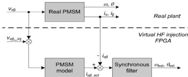
Fig1: Fundamental block diagram of VHFIM method
