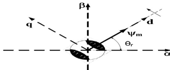
Fig2: definition of the dq and  $\alpha\beta$ -reference frame
