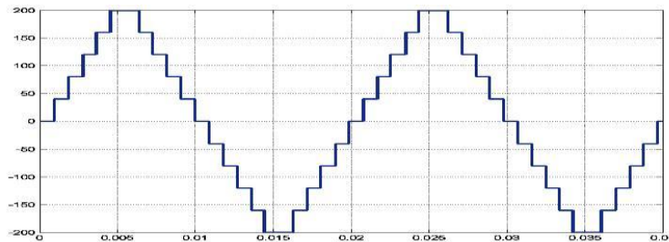
Figure 4: eleven level output of cascaded inverter
