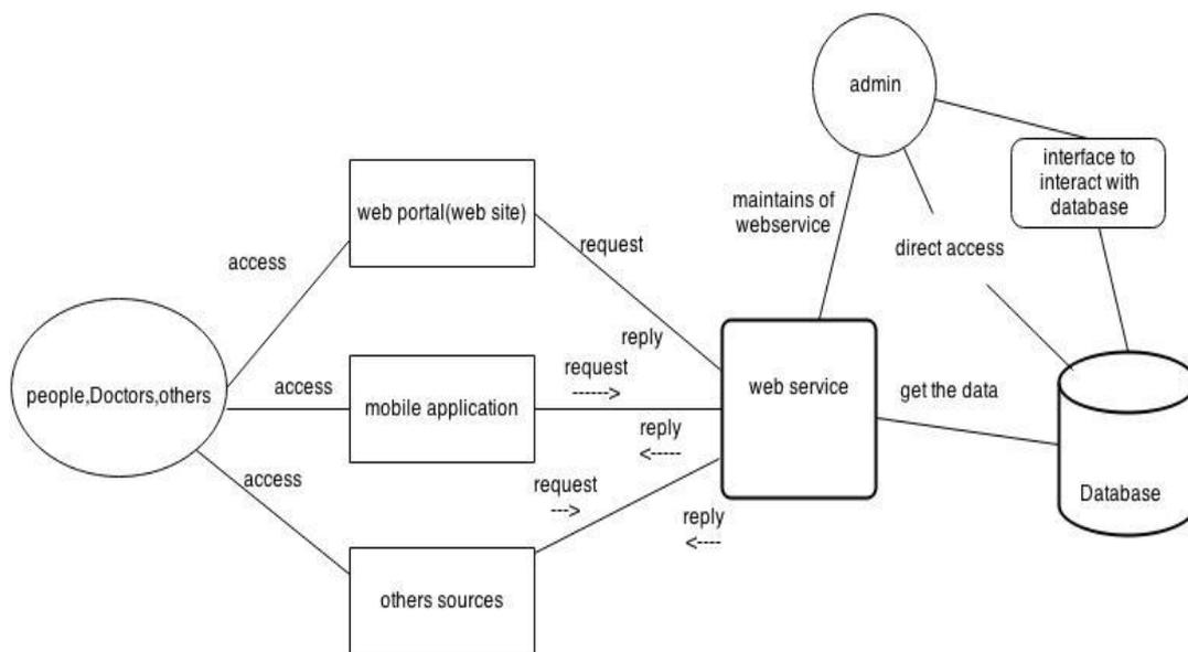
Figure: Architecture of proposed system.
