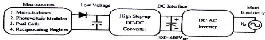
Fig.1. Basic schematic of microgrid consisting of microsources and power converters.
