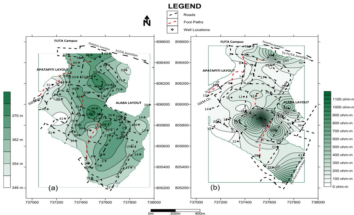
Figure 9: Comparison of groundwater elevation (a) and aquifer resistivity (b) maps
