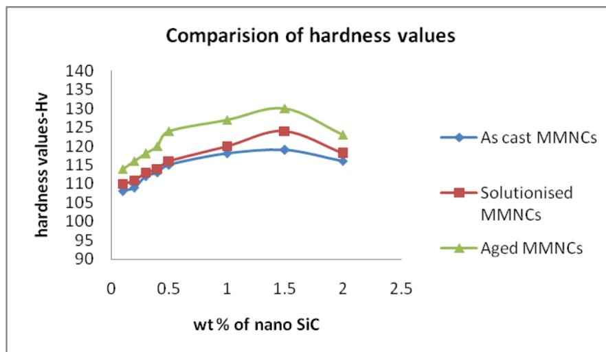
**Fig.3.** Hardness values of MMNCs for various wt% of nanoSiC<sub>p</sub>
