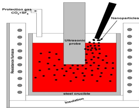
Fig.1. Sonicator with furnace
