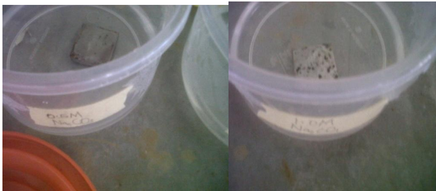
Fig 3 0.5M and 1.0M solution of Na 2 CO 3 with coupons immersed
