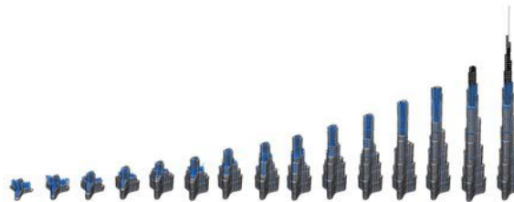
(a) Step by step of Model of construction sequential analysis of Burj Kalifa
