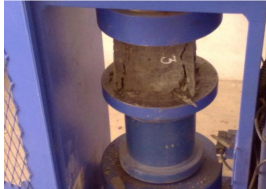
Fig 5: Testing of air entrained concrete Cube specimen
