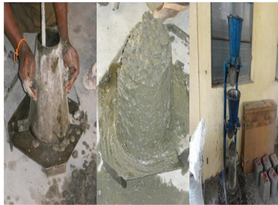
Fig 4: Measurement of Workability by Slump Cone and Compaction Factor apparatus
