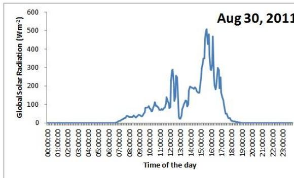
Figure 16: Diurnal plot of Global Solar Radiation for August 30, 2011
