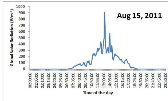
Figure 15: Diurnal plot of Global Solar Radiation for August 15, 2011
