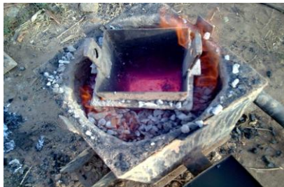
Fig. 6: Picture showing molten aluminium and water-cooled air inlet pipe
