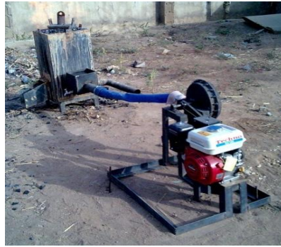
Fig. 5: Engine-driven blower being tested with an improvised charcoal fired furnace
