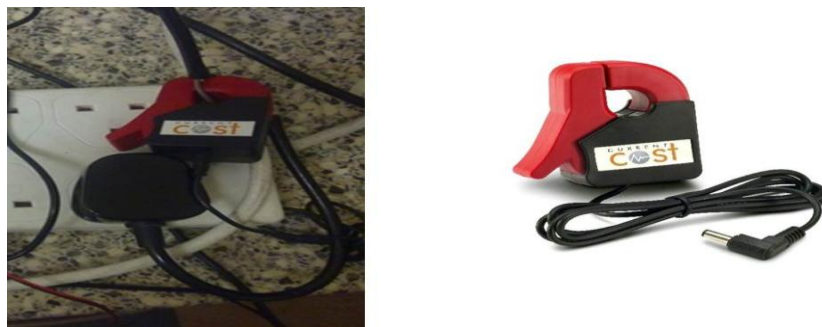
Figure 6 Current Sensor Based on Hall Effect
