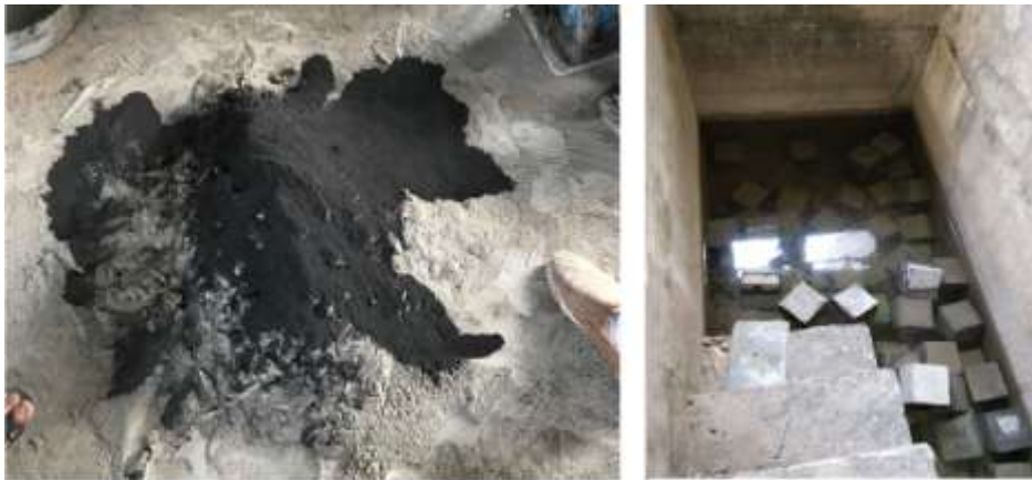
Fig. 1: Mixing of material to prepare the specimens and curing of specimens in tank
