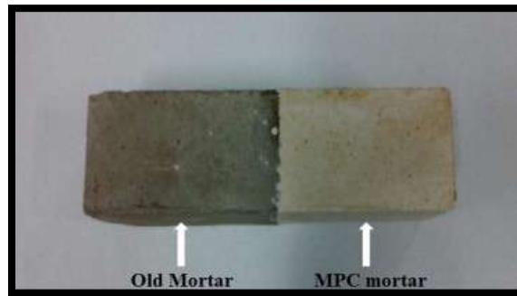
Figure 2.5: Ordinary and MPC mortar
