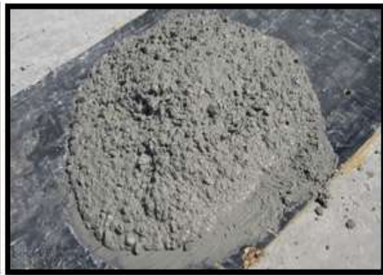
Figure 2.10: Fresh Silica Fume Concrete
