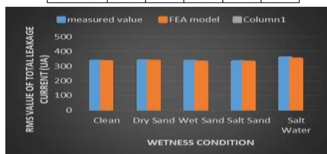
Figure 10: Comparison of RMS value of total leakage current between measurement and FEA model under different artificial pollution conditions.
