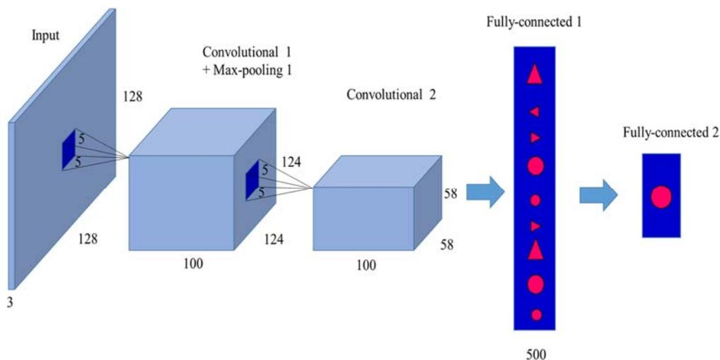
**Fig. 8 Proposed CNN architecture of face detection.**
