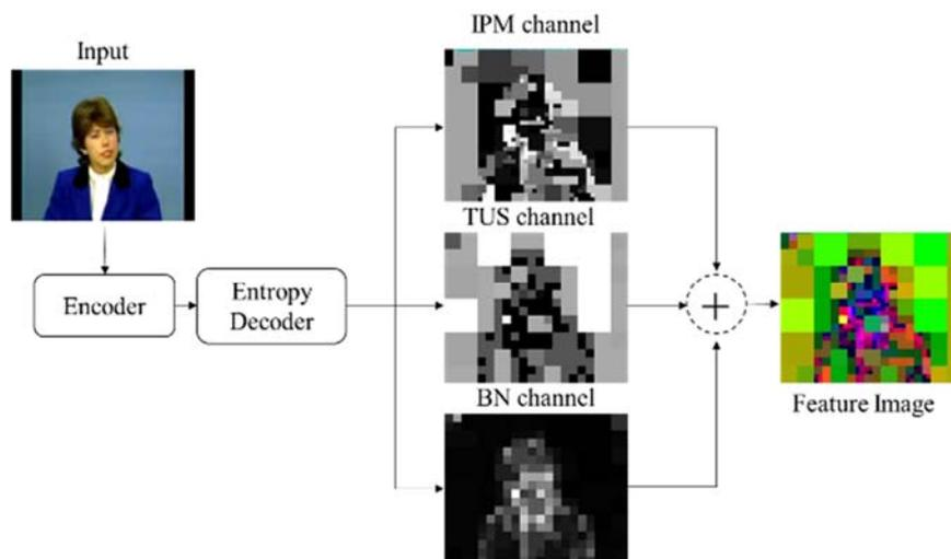
Fig. 7 Constructing feature image.
