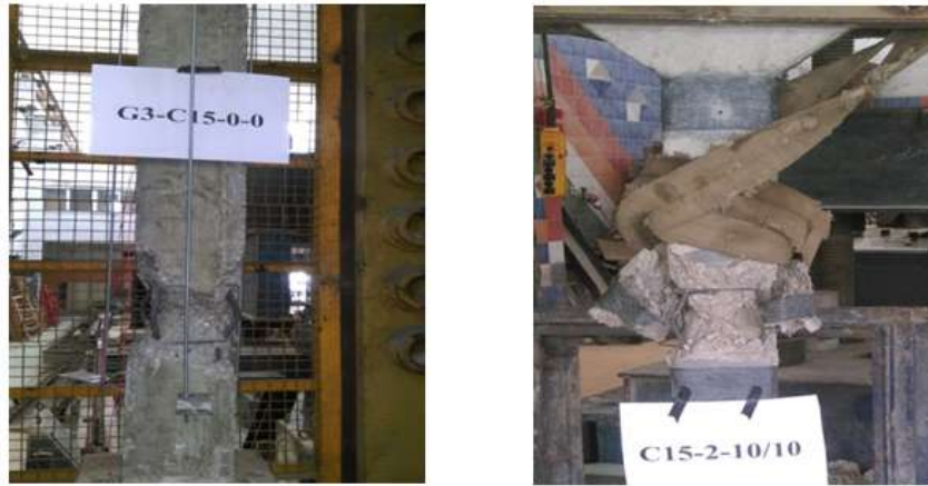
The Compression failure The Rupture of CFRP failure Fig.5: Different failure modes
