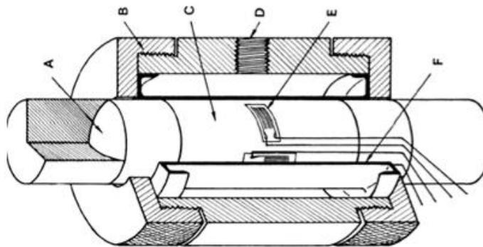
A- Spherical seat, B – Mild steel cell body, C – Rock specimen, D – Oil inlet, E – Strain gauges, F – Sealing membrane
