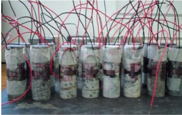
Figure 2: Specimens with strain gauges and lead-wires.
