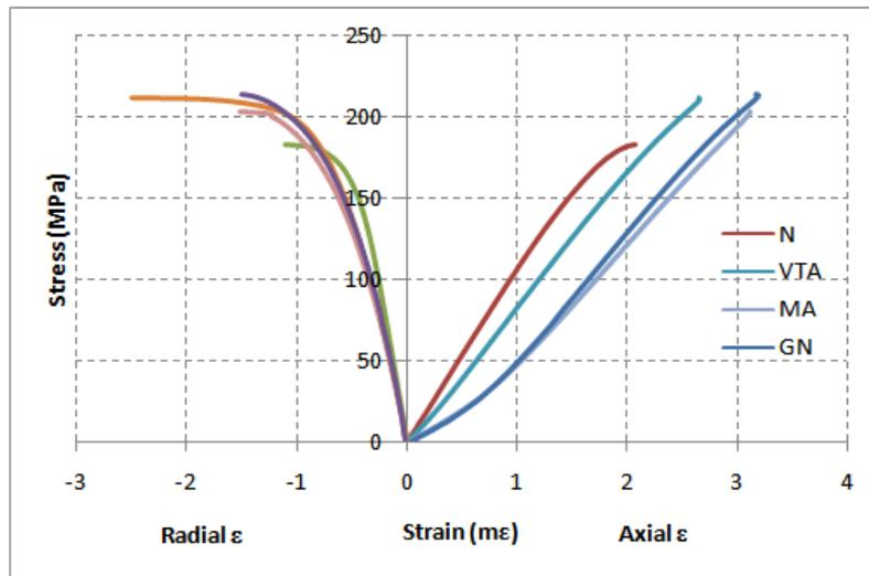
Figure 5: Stress-strain plot for Khomanani specimens
