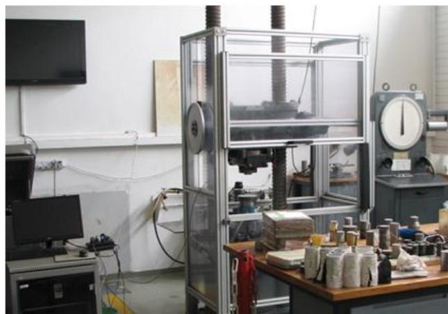
**Figure 1.** Amsler Compression Testing Machines
