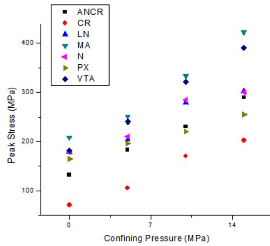
Figure 7: Plot of peak stresses versus confining pressures
