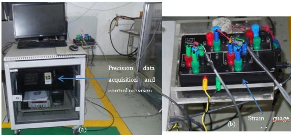
Figure 3: Data acquisition system (a) data acquisition and control unit (b) strain gauge amplifier.
